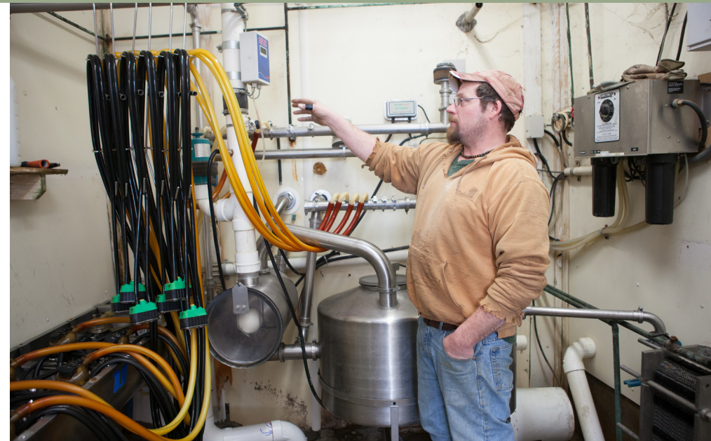
Alex explaining how the variable frequency holds the vacuum level on his milk pump.
