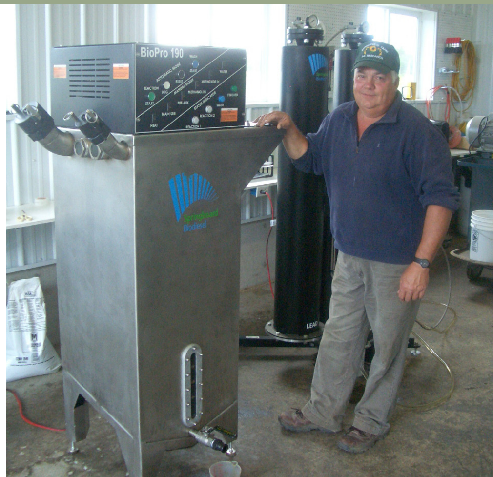
Roger Rainville with BioPro 190 automated biodiesel processor at Borderview Farm.
